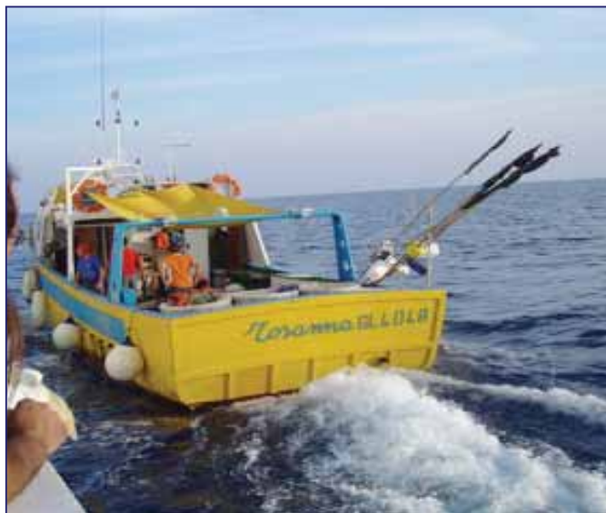
Fig. 2. The long-line fishing vessel, the 'Rosanna', used in the long-line surveys in the Santa Maria di Leuca coral region. (Home port Santa Maria di Leuca, roll GL 4048, length 14.10m, GRT 8.97tons, engine power 104.41kW.)
